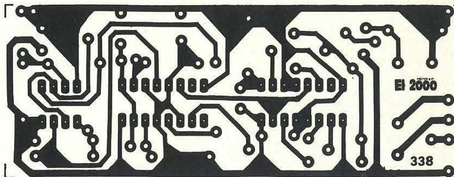
COMPONENTI - R1-R2 = 120 Kohm, R3-R4 = 150 Kohm, R5 = 1 Kohm trimmer, R6-R7 = 150 Kohm, R8 = 100 Kohm, R9 = 10 Kohm, C1-C2 = 10  $\mu$ F 16 VL, C3 = 3,3  $\mu$ F 16 VL, C4 = 100 nF, C5 = 220  $\mu$ F 16 VL, D1-D4 = 1N4148, D5 = 1N4001, T1 = BC108B, U1 = 1458, U2 = 4538, U3 = 4029, FR1-2 = Fotoresistenze, RL1 = Relé 12 volt. La basetta stampata, cod. 338, costa 5 mila lire.
