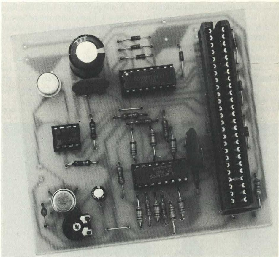
**COMPONENTI:** R1 = 75 Kohm, R2-R8 = 150 Kohm, R9-R13 = 75 Kohm, R14 = 5 Kohm trimmer, R15 = 750 Kohm, R16-R18 = 120 Kohm, R17 = 10 Kohm, C1-C4-C6 = 100 nF, C2 = 10 µF 16 VL, C3 = 1 nF, C5 = 100 µF 16 VL, U1 = 40174, U2 = L123, U3 = LF355, U4 = 4049, T1 = 2N1613, D1-D10 = 1N4148. La basetta, cod. 334, costa 6 mila lire.
